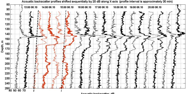
Acoustic backscatter profiles shifted sequentially by 20 dB along X-axis (profile interval is approximately 30 min)
