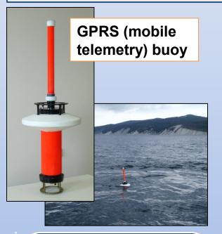
3. The GPRS buoy serves for the data and command exchange between the mooring and a user via Internet.
