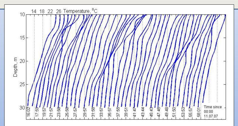
Sequential vertical profiles of the temperature are shifted by 2°C along X axis. Lower part from 30 m to 250 m is not shown.
