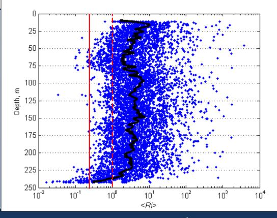
The mean gradient Richardon number  $\langle Ri \rangle = \langle N^2 \rangle / \langle U_z^2 \rangle$  as estimated from the profiler data on July 11-13, 2007. The thick black line is the vertical profile of the median values  $\langle Ri \rangle$ . Red line indicates  $\langle Ri \rangle = 0.25$ . Red dotted line indicates  $\langle Ri \rangle = 1$ .
