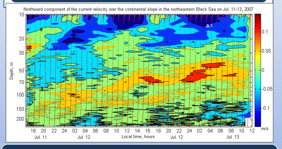
Example: Northward component of the current velocity over the continental slope in the northeastern Black Sea in July 2007. Thin red lines indicate location of the profiler during the survey.
