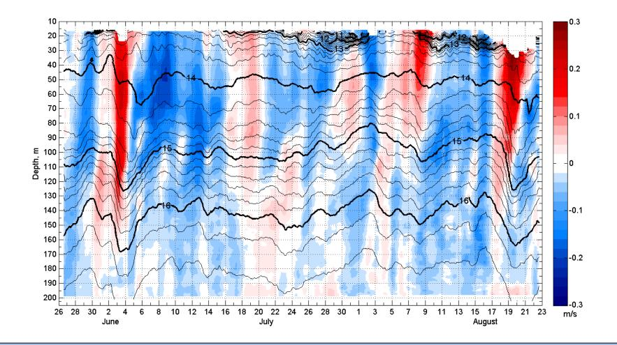
The potential density isopycnals (black lines) are superimposed on the time-depth diagram of the current variations .
