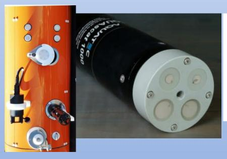
The AQUAscat transmits pulses of high frequency sound on 4 transducers, each of which may operate at a different frequency in the range from 500 kHz to 5 MHz. It measures the sound scattered by sediment or other suspended materials at discrete spatial intervals programmable from around 2<sup>1</sup>/<sub>2</sub> millimetres to several centimetres.
