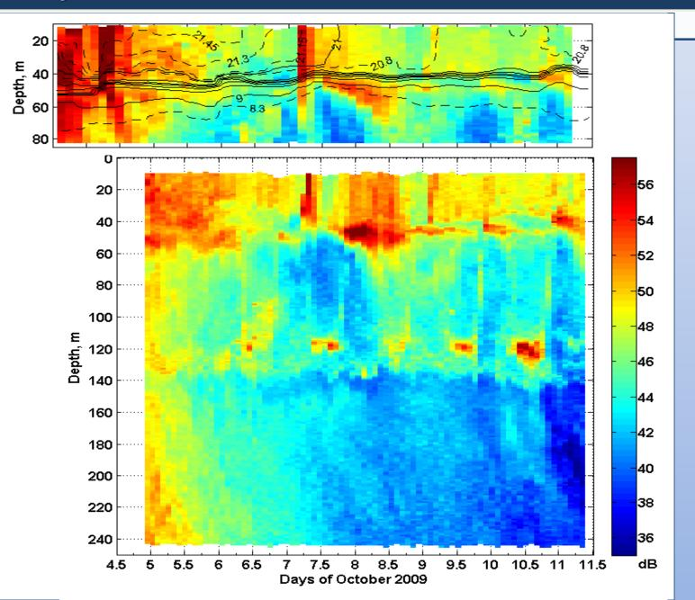
Variability of the acoustic backscatter at 2MHz at the coastal shelf break moored site during the survey and the vertical profiles of dissolved oxygen, fluorescence and turbidity as of October 4, 2009
