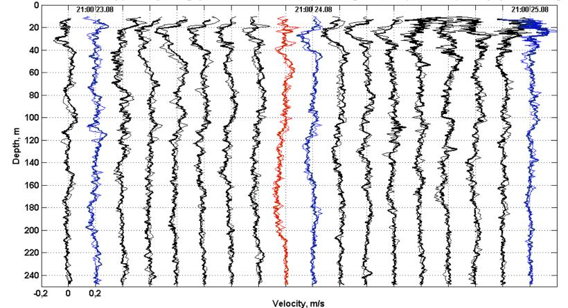
Cross-shels current velocity profiles (profiling cycle interval is 3 h since 18 p.m. of August 23, 2010) shifted sequentially by 0.2 m/s along X-axis
